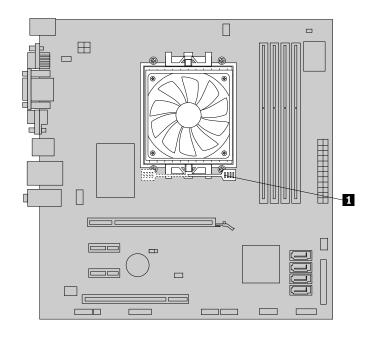
Figure 32. Reinstalling the heat sink and fan assembly
